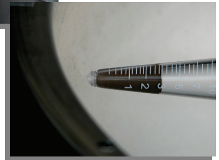
Conical shape of tube accentuates relatively small amounts of solids concentrations – as low as 00.20%.
