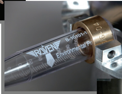
Tubes at full 90-degree angle to axis of rotation.
